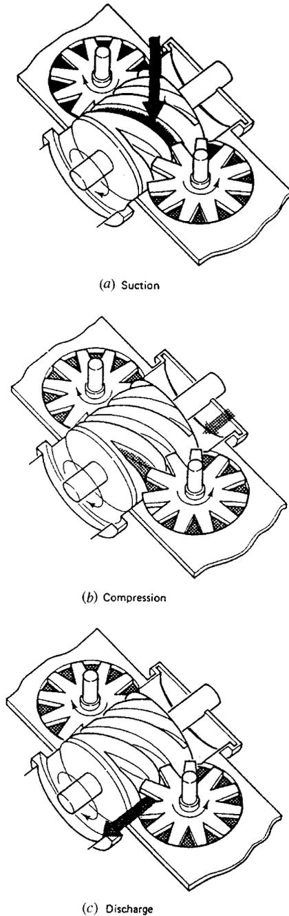
**Fig. 61.4** Diagram showing the operation of the rotary, single-screw compressor.<sup>1</sup>
