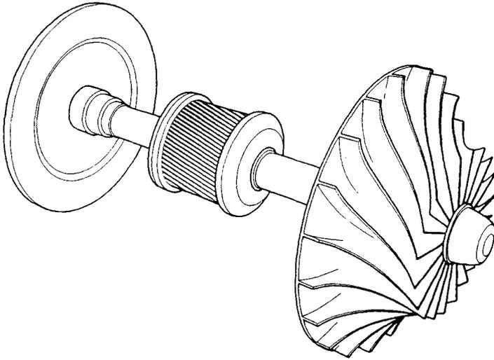
**Fig. 61.6** Pinion of an intergear unit having open, backward-curve-bladed impellers.<sup>1</sup>
