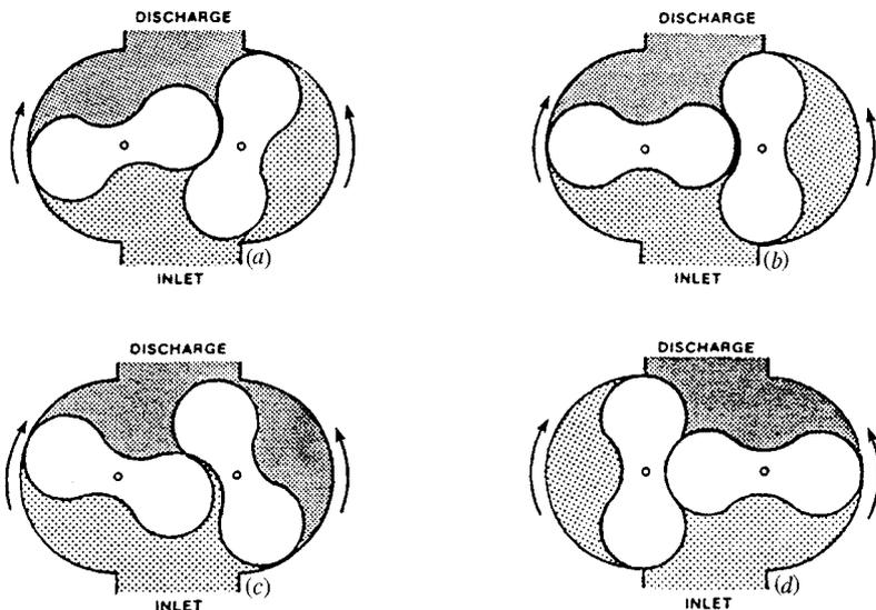
Fig. 61.9 Operating cycle of a straight-lobe rotary compressor (modified; courtesy of Ingersoll-Rand).<sup>2</sup>
