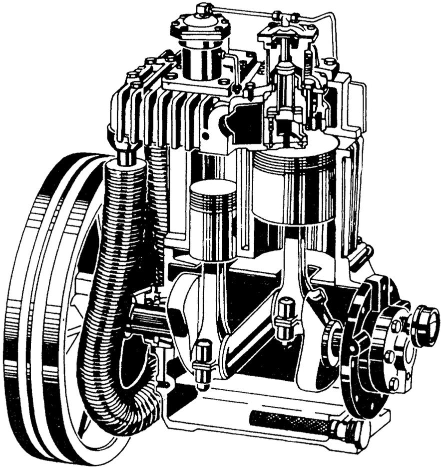
Fig. 61.2 Single-acting, two-stage compressor.<sup>1</sup>
