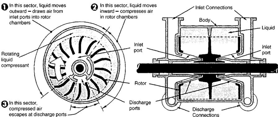
Fig. 61.10 A sectional and end view of a liquid ring compressor (courtesy of Nash Engineering Co.).<sup>2</sup>
