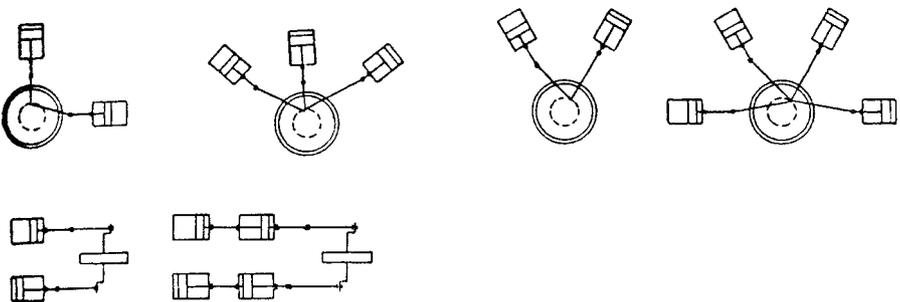
**Fig. 61.3** Various cylinder arrangements used in displacement compressors. Some are suitable for single-acting compressors, while others are double-acting and require a crosshead and guide.<sup>1</sup>
